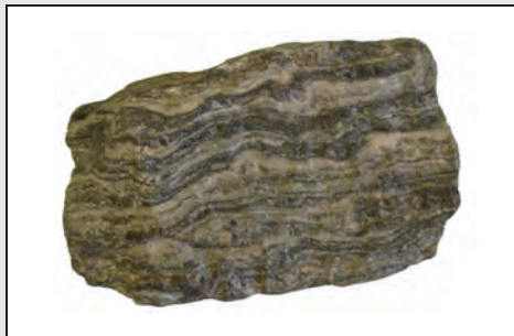
Gneiss —originally igneous or sedimentary. The bands are caused by high shear forces that cause the rock to behave like plastic. (Photo courtesy of Siim Sepp 2005, CC BY-SA 3.0.)
